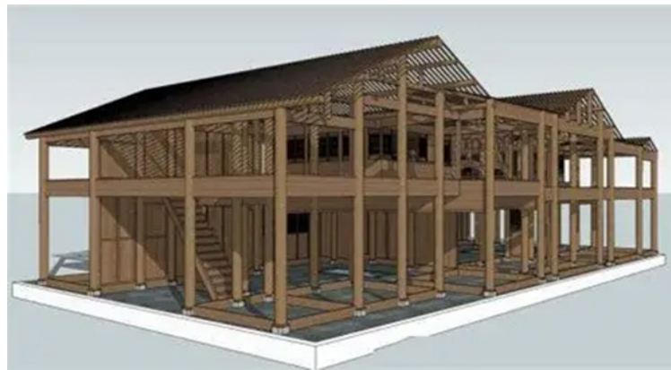
Figure 6. Translation in the Arrangement of Structural Columns
